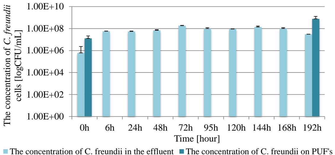
Fig. 2. The concentration of *C. freundii* cells (immobilized on PUFs) before, during and after bioconversion process (average values of triplicates).
