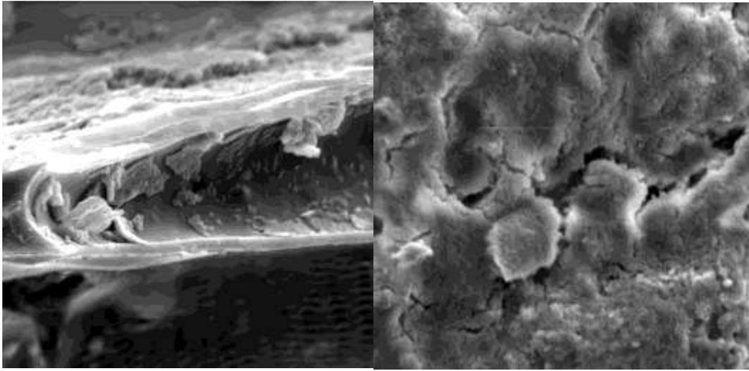
Fig. 1. Adhesion of *C. freundii* cells to the surface of modified PUFs (left) and keramsite (right).
