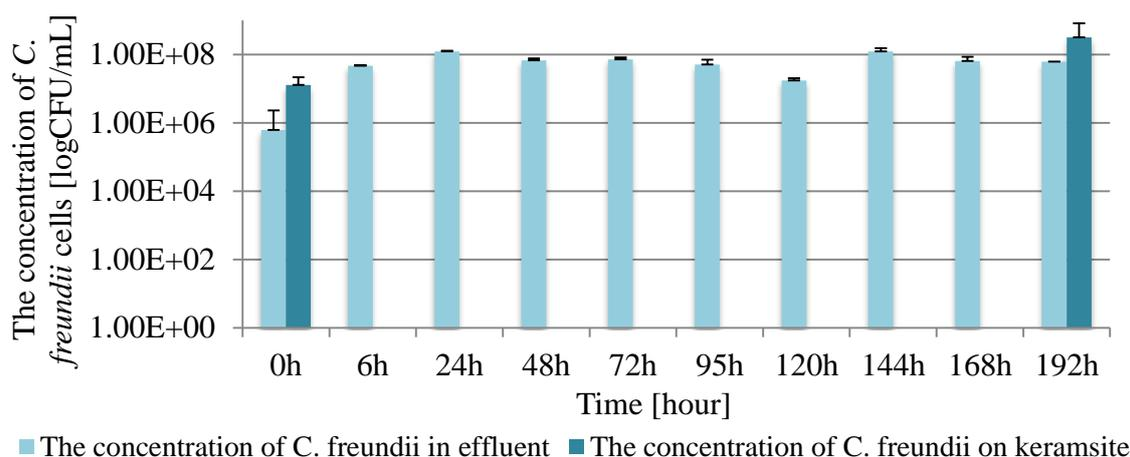
Fig. 3. The concentration of *C. freundii* cells (immobilized on keramsite) before, during and after bioconversion process (average values of triplicates).
