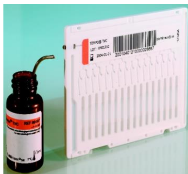
Figure 2. Card with a transfer tube and an ampule with a specific culture medium.
