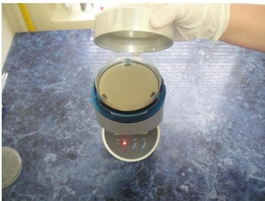
Fig. 5. Equipment for sampling air (placing the Petri plate which contains culture medium)
