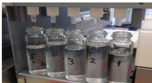
Fig 5. Purification of the supernatant through the florisil cartridge
