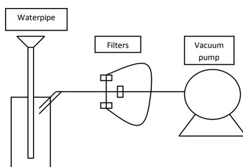
Figure 1. Schematic of system set for collecting WTS
