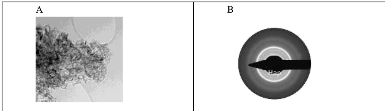
**Fig. 3. TEM (a) image and SAED (b) pattern for Hap substituted with zinc ions powder, annealed at 500°C/2h**
