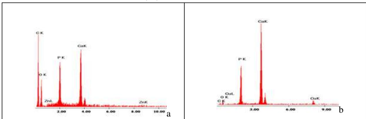
**Fig. 5 EDAX spectrum of Hap substituted with zinc (a) and copper ions (b)**
