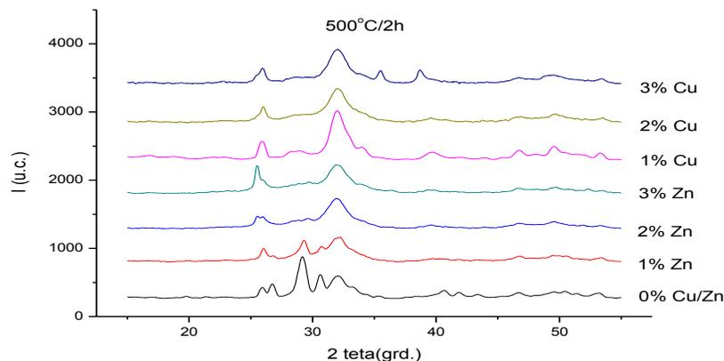
Fig. 1. XRD pattern of the unsubstituted sample and for samples substituted with zinc ions and with copper ions, annealed at 500°C/2h
