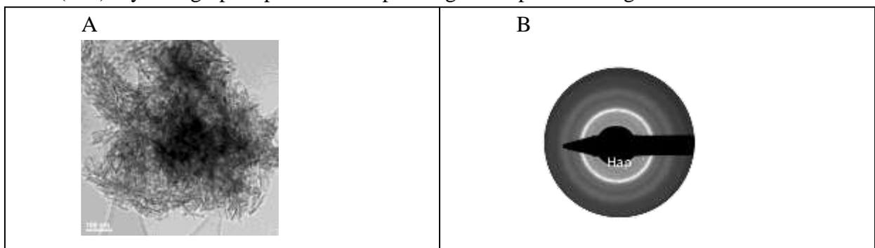
**Fig. 4. TEM (a) image and SAED (b) pattern for Hap substituted with copper ions powder, annealed at 500°C/2h**
