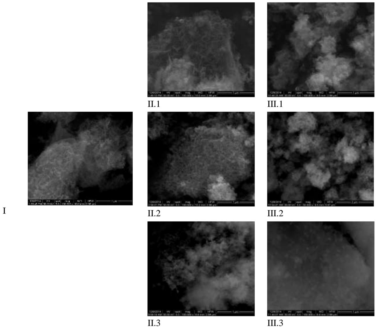
Fig. 2. SEM images for the unsubstituted sample and for samples substituted with zinc ions and copper ions, annealed at 500°C
