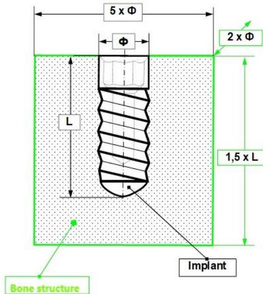
**Figure no. 5.** 3D model of the studied periimplantation area.
