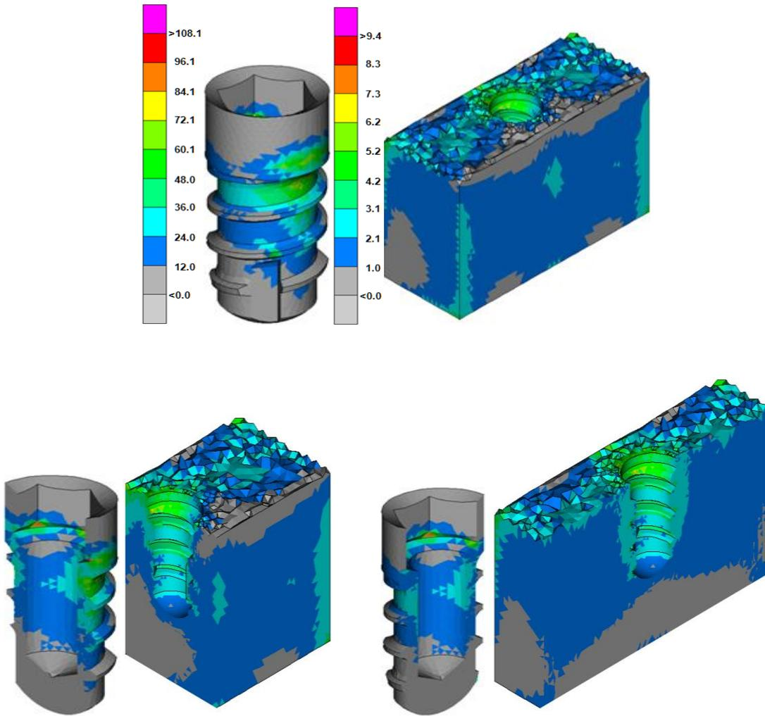
**Figure no. 11.** Von Mises equivalent stress distribution for Titanium implant,  $\Phi = 3.6$  mm;  $L = 9$  mm, at an action of the masticatory force under an angle of  $90^\circ$  considered linguo-vestibular. Maximum Values  $\sigma_{VM}$ : Implant  $\sigma_{VM} = 108.1$  [Mpa]; Mandible  $c_{VM} = 9.4$  [Mpa].
