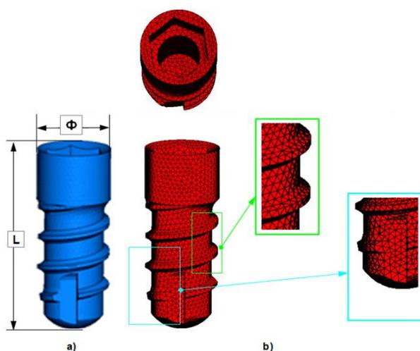
**Figure no. 4.** 3D model of the type 2 implant (a) 3D model; (b) 3D mesh model.
