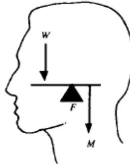
**Figure no. 1.** Forces and Supports - First-degree lever (NASA [19]).
