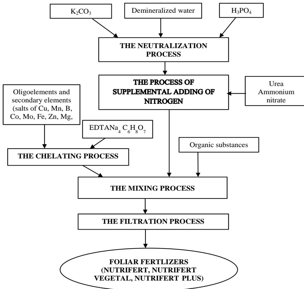
**Figure 1.** Technological flow of production of NPK liquid fertilizers with secondary nutrients and trace, and organic substances
