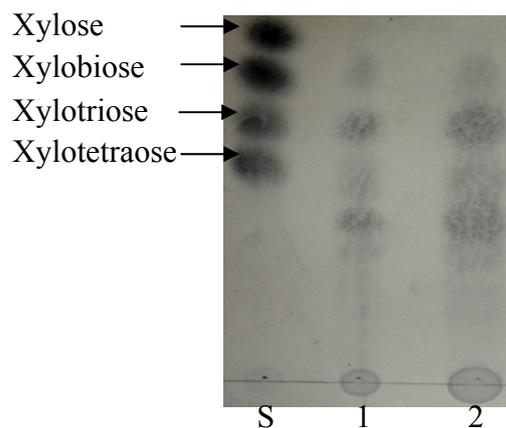
**Figure 3.** Thin layer chromatography of xylan hydrolysis products by XynA16. Lane S: Xylose standards, Lane 1: products of 1 h enzymatic reaction, Lane 2: products of 2 h enzymatic reaction
