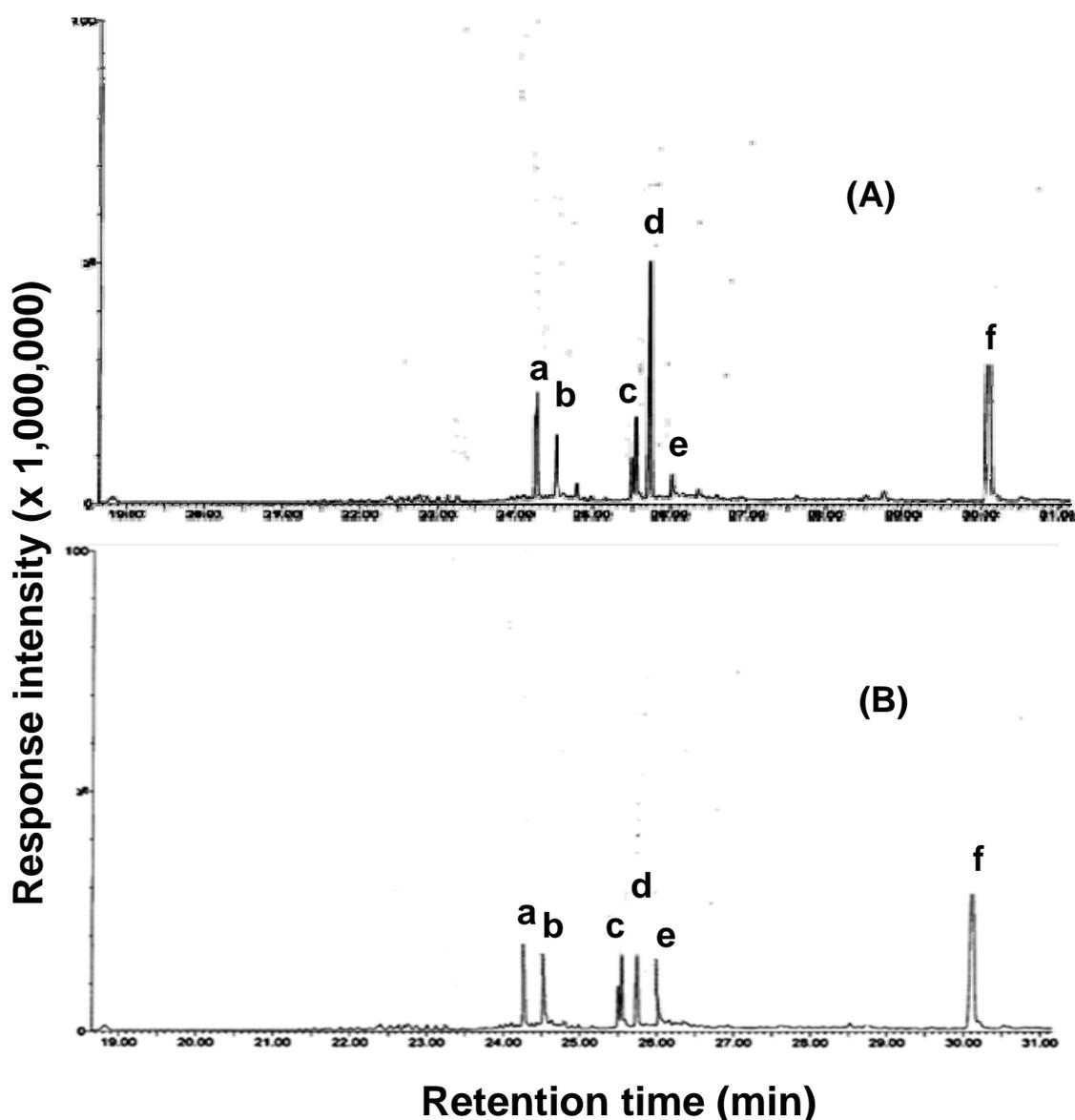
**Figure 5.** Gas chromatographic profile of fatty acids of *Basella alba* seed oil. (A): oil sample; (B): standard fatty acids. (a): palmitic acid; (b): stearic acid; (c): oleic acid; (d): linoleic acid; (e): linolenic acid; (f): erucic acid (internal standard)
