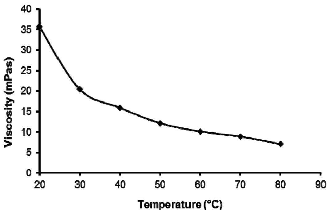
**Figure 1.** Effect of temperature (20-80 °C) on *Basella alba* seed oil viscosity
